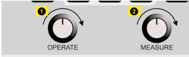
1. OPERATE knob. Runs a breaker operation sequence without measurement.
